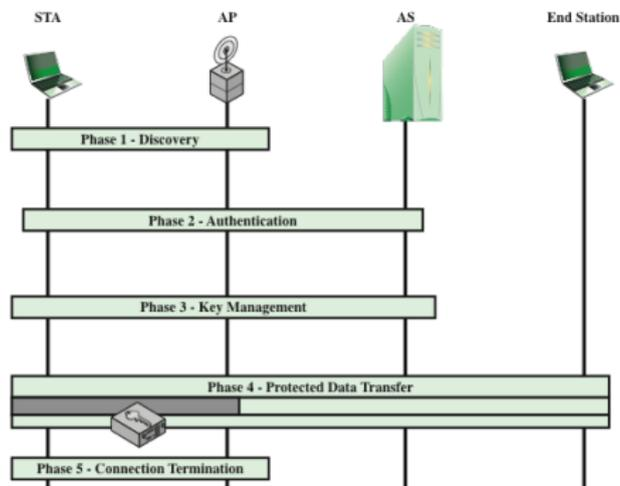
Figure: 802.11i Phases of operation [1]
