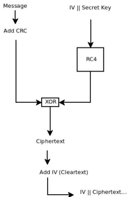
Figure: WEP encryption process
